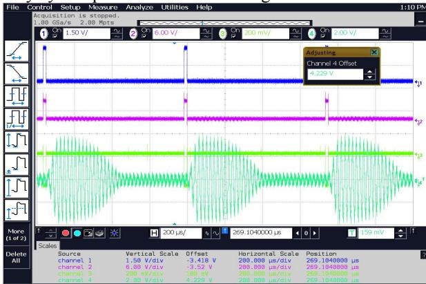
Fig.11. Beam current, Detected RF and inverter Current Waveforms
